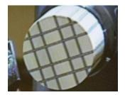
She alternates 3 black veneers with two natural ones and sandwiches them between planed blocks using Titebond PVA to glue them all together. She then slices the block at right angles to the veneer and adds more veneer in between the cut surfaces and ends with a chequered effect.
