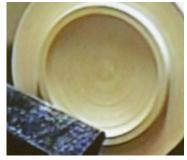
The inside diameter of the bowl was measured, and the measurement transferred to the lid blank. Carlyn then turned the wood away that was outside of the mark to a depth such that the lid would sit securely on top of the bowl. She then hollowed out the inside of the top to a shallow depth. She checked the fit with the bowl and then reduced the overall diameter so that when fitted the lid would overhang the bowl by a short distance.
